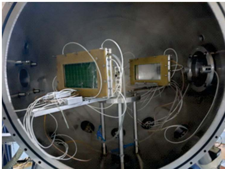
Fig. 5.1.15.1: Experimental setup with two MWPCs placed at 154° folding angle and two Passivated Implanted Planar Silicon (PIPS) detectors at 15° with respect to the beam direction.
