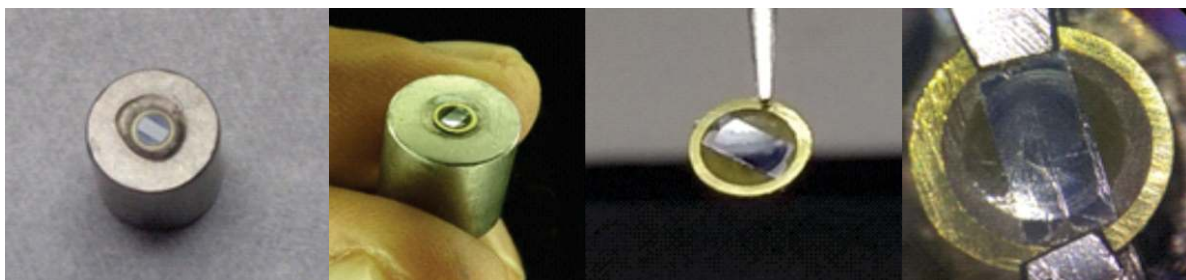
Fig. 4.4.4.2: Glimpse of XTEM sample preparation using a strip of the sample
