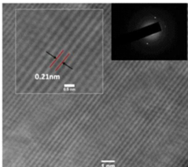
**Fig. 3:** HRTEM image of the  $\text{MoS}_2$  thin film. An interlayer distance of 2.1 Å is assigned to the (100) plane of  $\text{MoS}_2$  [Budhi Singh et al, *Mater. Res. Express* 6 (2019) 096424]
