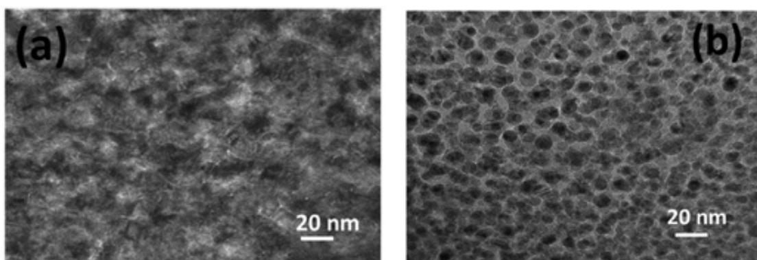
**Fig. 5:** (a) TEM image of as deposited, and (b) TEM image of ion irradiated thin film [Deepthi et al, *Sensors & Actuators: B. Chemical* 301 (2019) 1270067]
