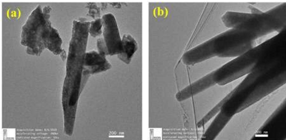
**Fig. 6:** TEM images of (a) pristine ZnO thin film and (b) 30 kGy gamma-irradiated ZnO thin film [Maqsood R.Waikar et al, *Journal of Alloys and Compounds* 830 (2020) 15464110].
