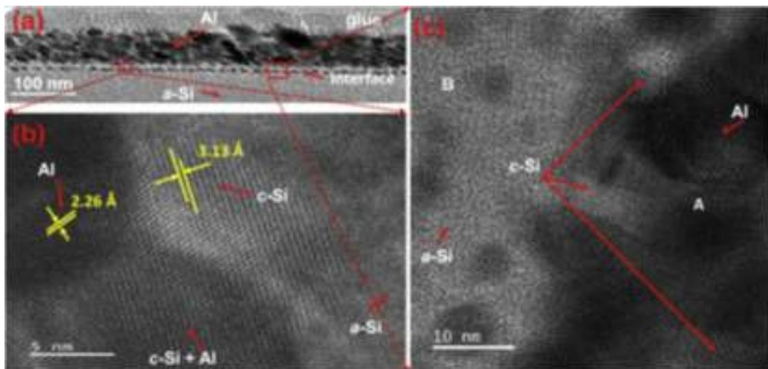
**Fig. 2:** (a) Cross-sectional TEM (XTEM) image of a typical sample irradiated with  $5 \times 10^{12}$  ions- $\text{cm}^{-2}$  and (b-c) high resolution TEM (HRTEM) images of the same sample [G. Maity et al, *Journal of Non-Crystalline Solids* 523 (2019) 119628].
