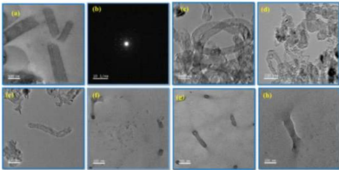
**Fig. 4:** The TEM images of (a) pristine MWCNTs, (b) SAED pattern of pristine MWCNTs, and (c)–(h) post  $\gamma$ -irradiated MWCNTs at 10–60 kGy doses [Maqsood R. Waikar et al, *Materials Science in Semiconductor Processing* 110 (2020) 104975].
