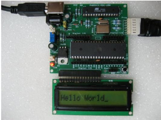
Figure 2.3: PMDK-USB with LCD Display
