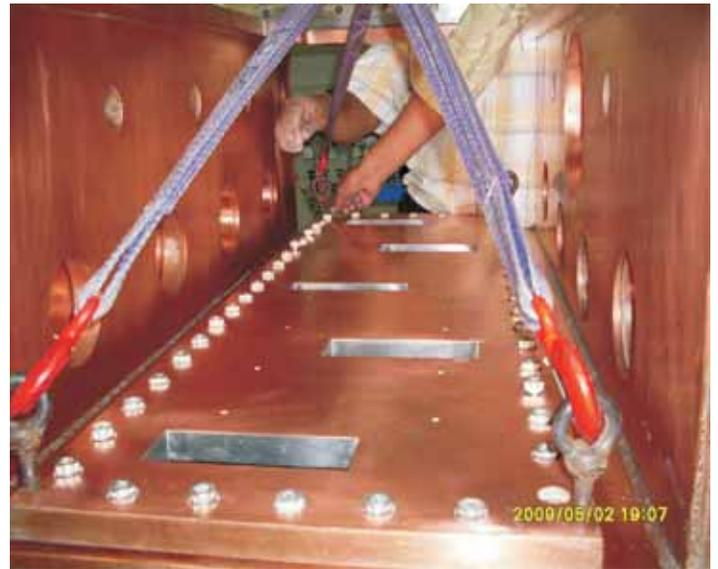
*Fig. 1. Copper plated prototype RFQ chamber*
