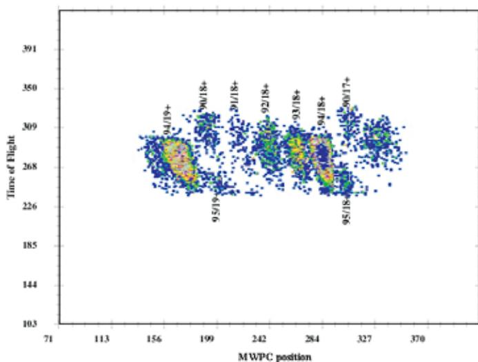
**Fig. 2** Position at focal plane ( $M/q$ ) versus  $(T_0\text{-TOF})$  for  $^{28}\text{Si}$  ( $97\text{ MeV}$ ,  $2\text{ microsecond pulse separation}$ ) on  $^{94}\text{Zr}$ ;  $M/q$  ambiguity is resolved and so are the transfer channels
