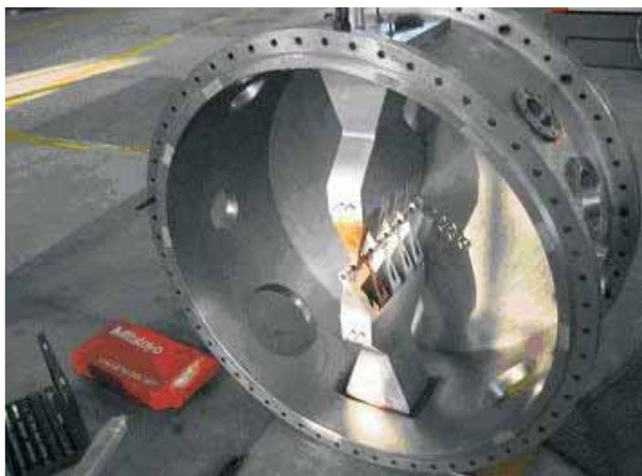
*Fig. 1 Prototype resonator with one end-plate removed*
