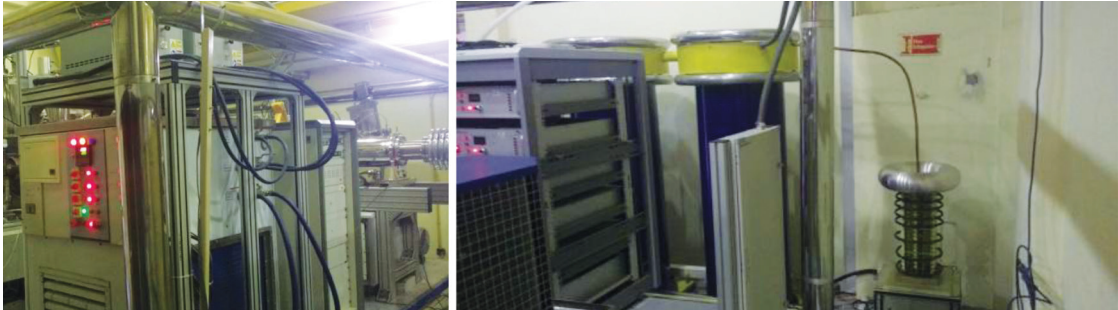
Figure 2.1.7. (Left) PKDELIS ECR Ion source on high voltage platform and (Right) HV platform power supply
