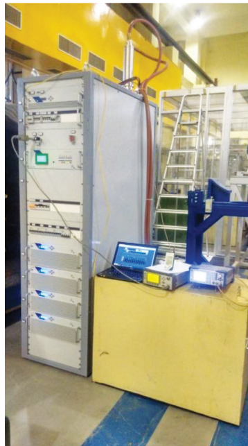
Fig.2.1.29 Burn-in Test at IUAC with 50 Ohm Load
