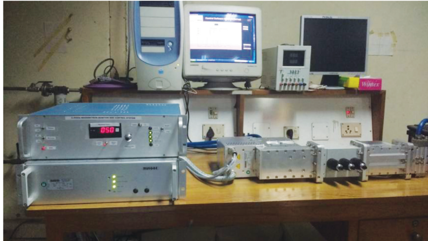
Figure 2.3.3. Testing of 1 kW microwave generator using indigenously developed controller
