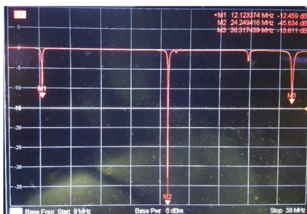
Figure 2.1.8 Tuned frequencies as seen on VNA
