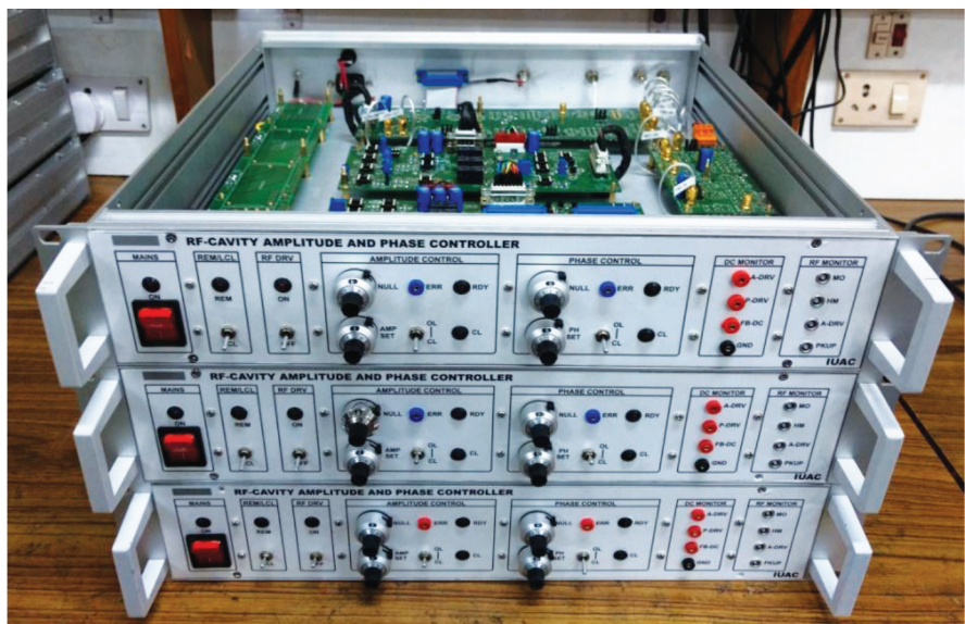
Figure:2.1.24 amplitude and phase controllers for the RF cavities.
