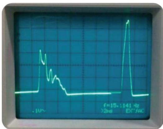
Figure 1.3.3 A typical beam profile of non-analyzed beam
