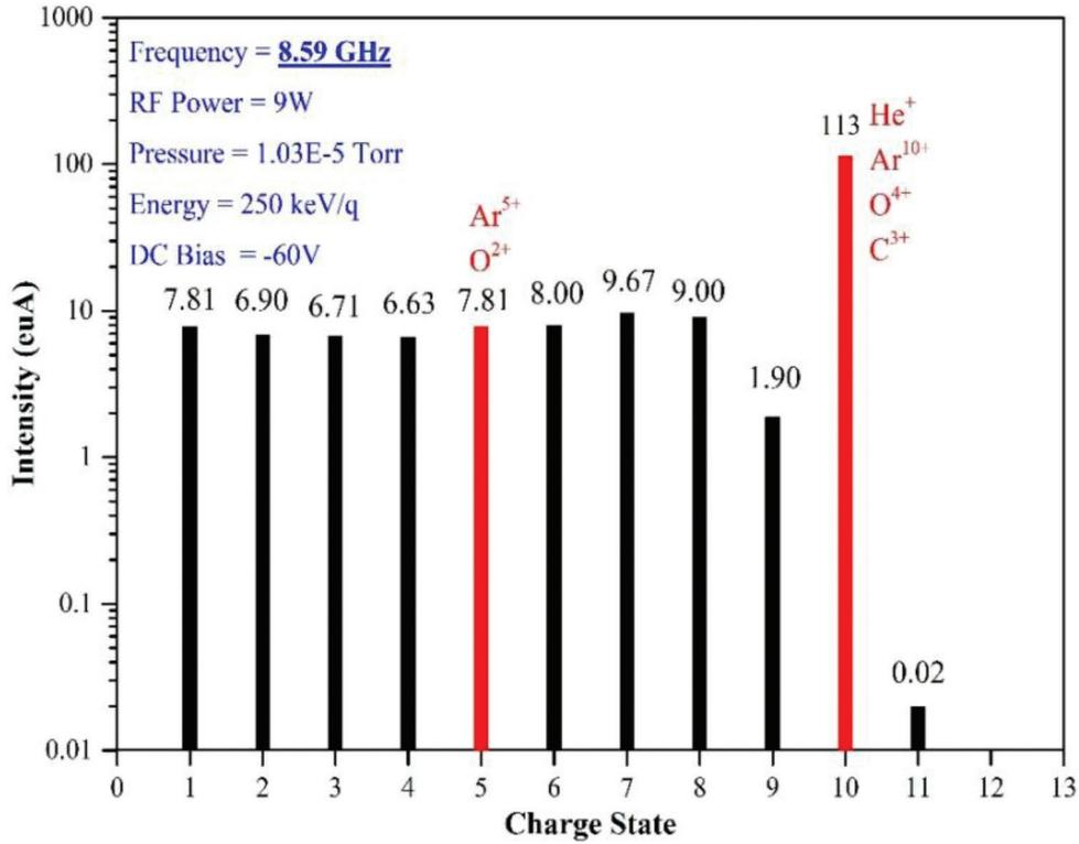
Figure 1.3.2 A typical charge state distribution of the argon showing the influence of the helium mixing on the higher charge states.
