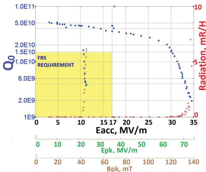
Figure 1.2.5: 2K Performance of the first 650 MHz,  $\beta=0.6$  single cell niobium LBC.
