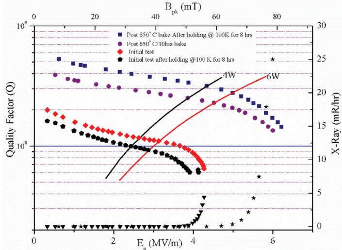
Figure 1.2.3: Q curves for the QWR pre and post 650°C bake.
