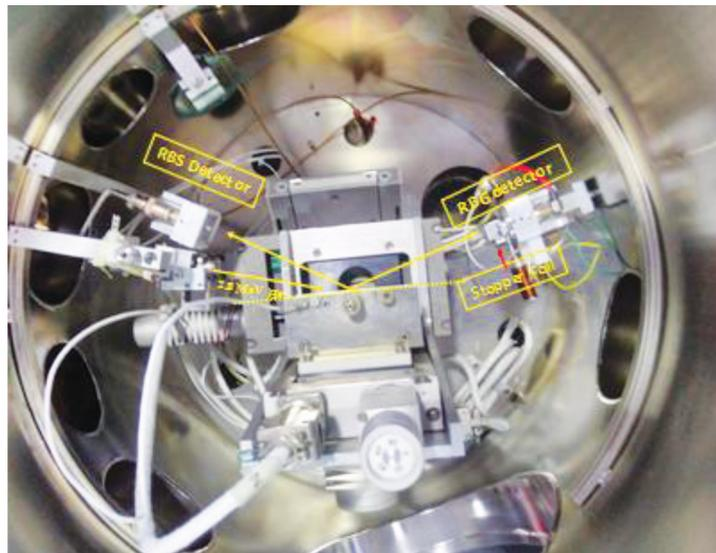
Fig 1.4.2 End station experimental chamber for RBS with ERDA(RBG) measurement setup
