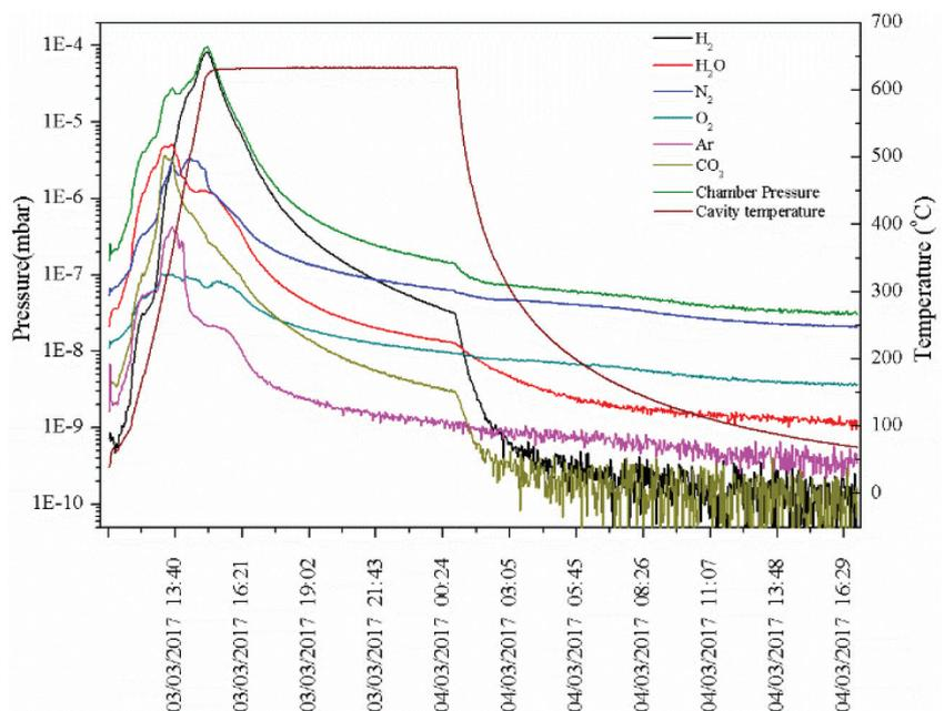
Figure 1.2.2: RGA spectrum during  $650^\circ\text{C}$  bake of the QWR.
