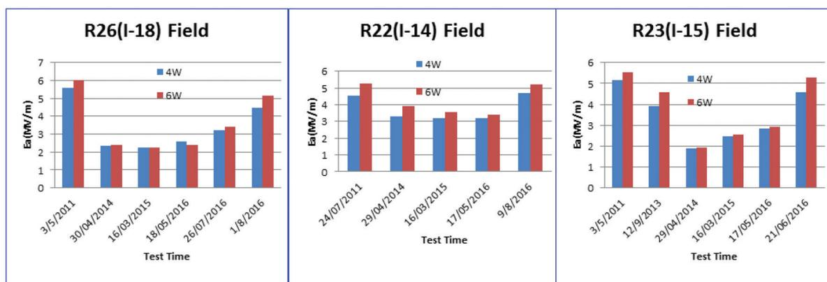
Figure 1.2.1. The accelerating field performances of three resonators during last few years. The last performance (in 2016) of all the three resonators were done in test cryostats and the remaining tests were done in the linac cryostat.
