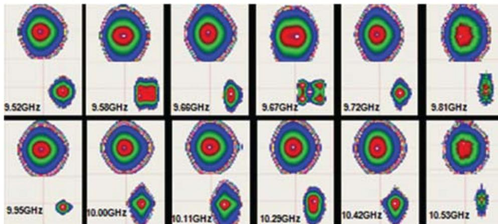
Fig. 5 The shapes of total and analyzed oxygen beams at the injection of different frequencies. The smaller shapes are of the analyzed beam ( $O^{+5}$ ).
