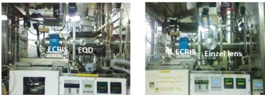
Fig. 7 Inside view of high voltage platform. The EQD (shown in left side image) has been replaced with Einzel lens (Right side image)
