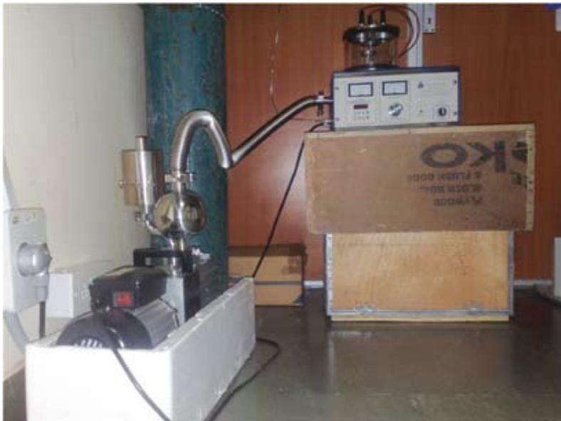
Fig. 8 Plasma coater for thin metallic film deposition
