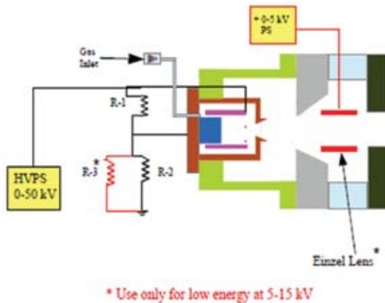
Fig. 11 Schematic diagram of PIG Ion Source
