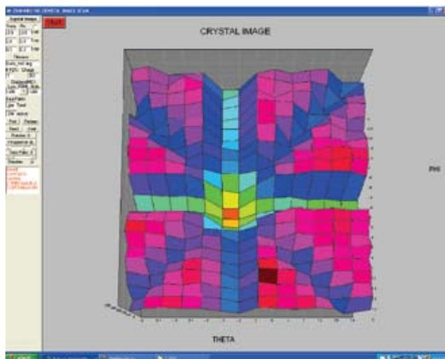
Fig. 1. Channeling image scan of GaAs ( 100) crystal
