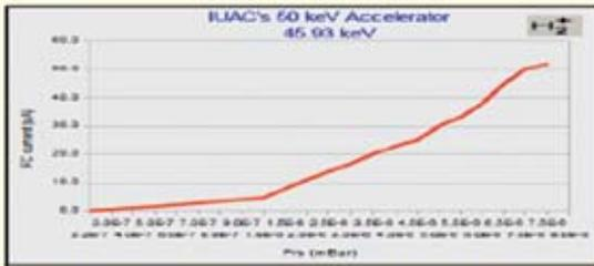
Beam Current Vs Source Prs. At 49 kV, 1721 G
