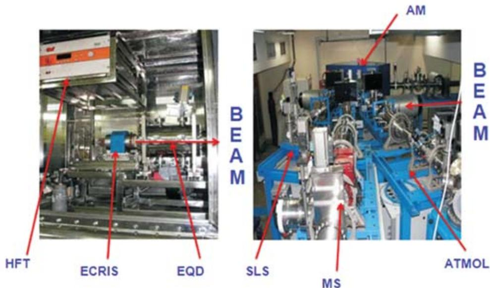
Fig. 1. All permanent-magnet-ECR source along with peripheral electronics on high voltage platform and view of the beam hall. HFT and AM stands for high frequency transmitter and analyzer magnet respectively. Others abbreviations used in the figure are already explained.
