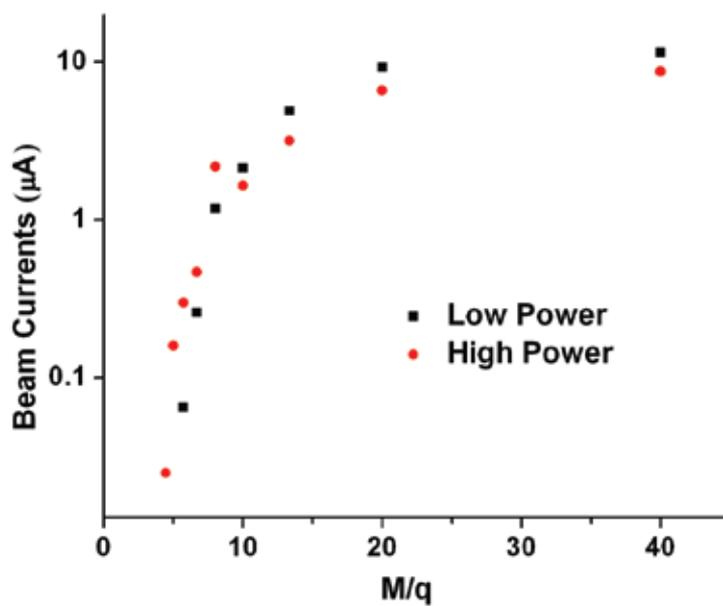
Fig. 3. Charge state distribution (CSD) of argon at  $E/q = 212$  kV and two power levels (2 and 70 watt).
