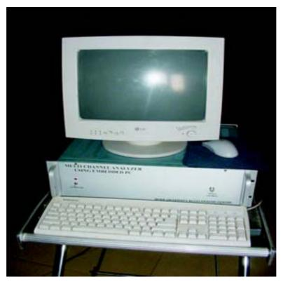
Fig.1. Portable Multi Channel Analyzer (MCA) system using Embedded PC
