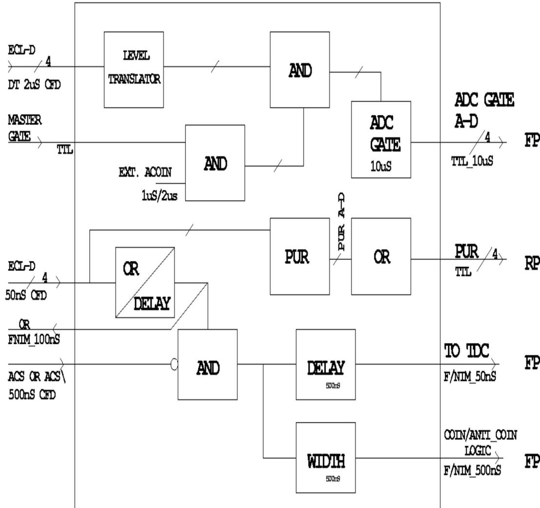
FIG: BLOCK DIAGRAM OF COIN/ANTI\_COIN LOGIC CIRCUIT
