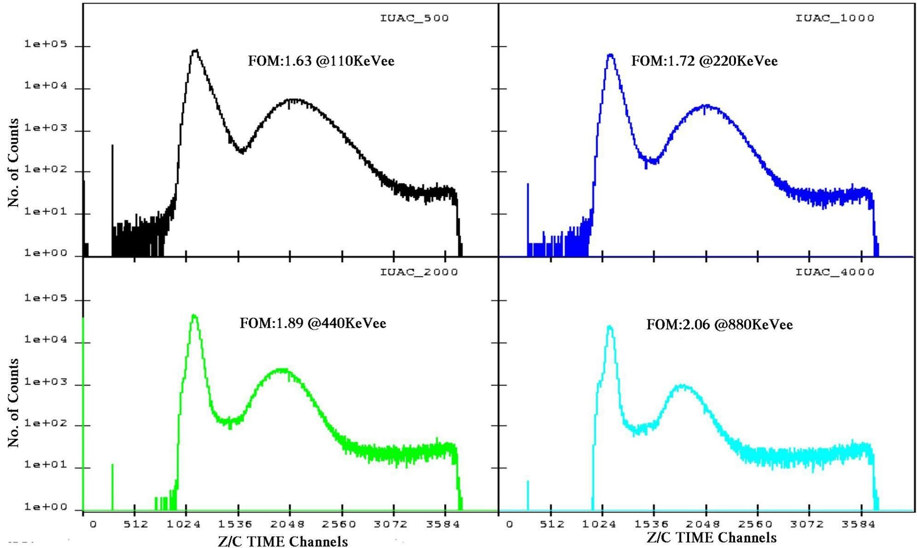
**Table: FOM obtained with PSD electronics at different energy thresholds compared with commercial and other arrays**
