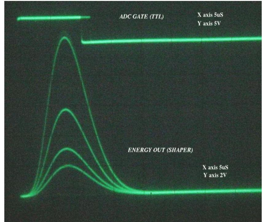
**ACLogic card, ADC Gate, Unipolar output**
