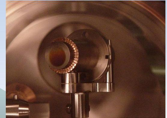
Cathode block with Cs<sub>2</sub>Te coating
