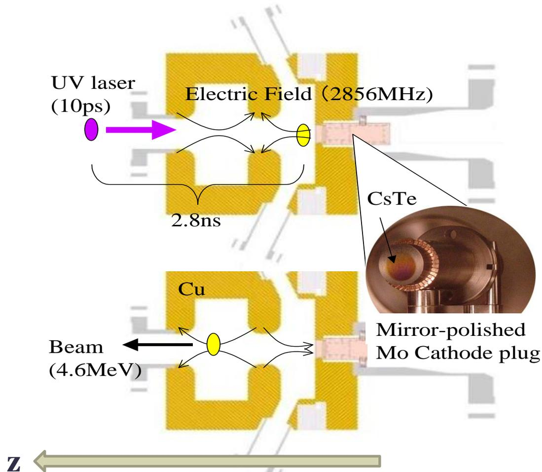
Laser pulse with the pulse duration of **10psec(FWHM)** is irradiated on  $\text{Cs}_2\text{Te}$  thin film photo-cathode. Figures show 1.6cell-2856MHz RF cavity and an electron bunch accelerated in the cavity.
