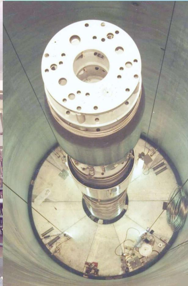
Accelerator tubes and equipotential rings installed
